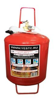
Powder fire extinguisher OP-25, pumped with extinguishing powder and gas (air, nitrogen, carbon dioxide) to a pressure of 16 atm.; fire extinguisher grade – 6A, 233B, weight of fire extinguishing powder – 25 kg, cylinder volume – 25 l, the supply time of the extinguishing agent is 20 seconds.
