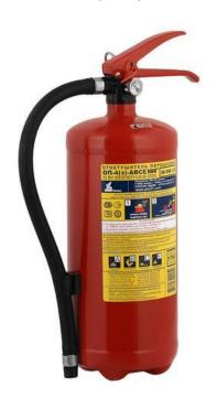
Powder fire extinguisher OP-4 (z)-AVSE 'MIG' with increased fire extinguishing capacity, pumped with dried nitrogen to a pressure of 16 atm.; fire extinguisher grade – 2A, 70B, C, E, powder grade – 'Vekson-ABC 25', weight of fire extinguishing powder – 4 kg, cylinder volume – 5 l, the supply time of the extinguishing agent is 10 seconds.
