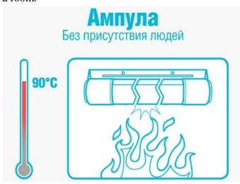
During a fire, as the temperature rises, a series of chemical reactions begin in the device, and as a result, pressure increases inside the ampoule. When the temperature of the extinguishing agent reaches 90 °C, the ampoule breaks down and sprays the contents over the source of ignition. In this case, most of the liquid passes into the gaseous phase.
